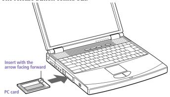
Do not force a card into the slot as this may damage the connector pins. If you have difficulty inserting a card, check that you are inserting the card with the correct orientation. See the manual that came with your PC card for more information on use.
